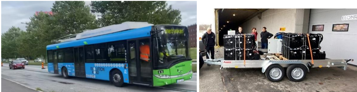
Figure 3-4 Left: A Nissan Leaf and a City bus drawing power at the same time Right: A dummy load trailer with pick up for the ERS
