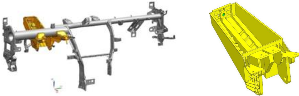
Figure6: Demo 3 - Cross car beam (left: benchmark product, right: new design) [12]
