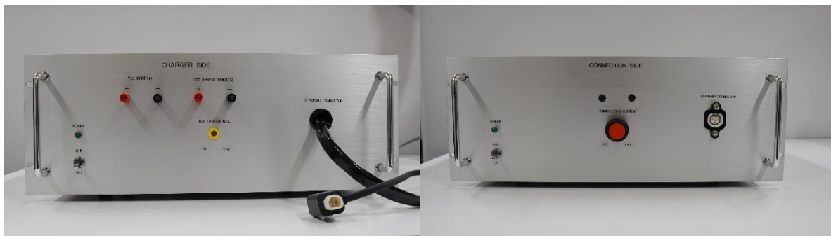
Figure 7: test-prototype of charger (left) and dummy battery (right)
