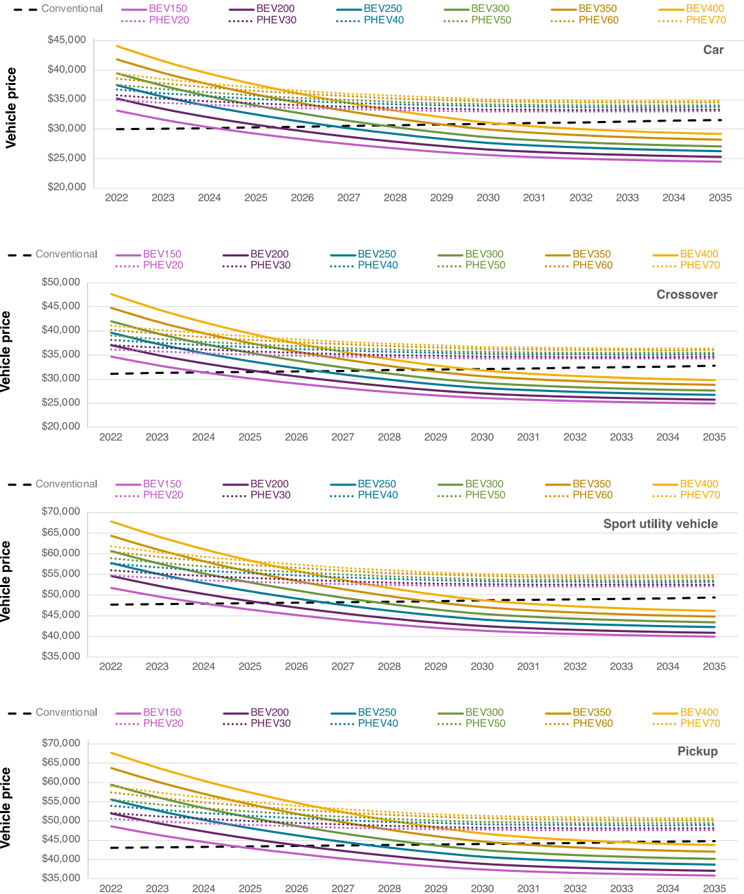
Figure 3: Initial price of conventional and electric vehicles for 2022–2035 for four vehicle classes
