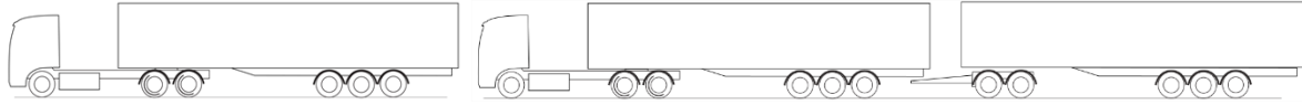
Figure 1. Tractor and semitrailer (prototype) with the nominal GVW 40t configuration (left) and a HCT configuration of tractor, semitrailer, dolly and another semitrailer with GVW of 76t (right).
