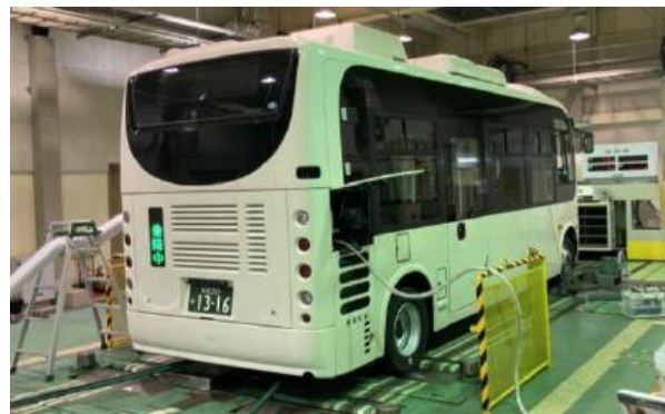
Figure 4: Vehicle during chassis dynamometer testing
