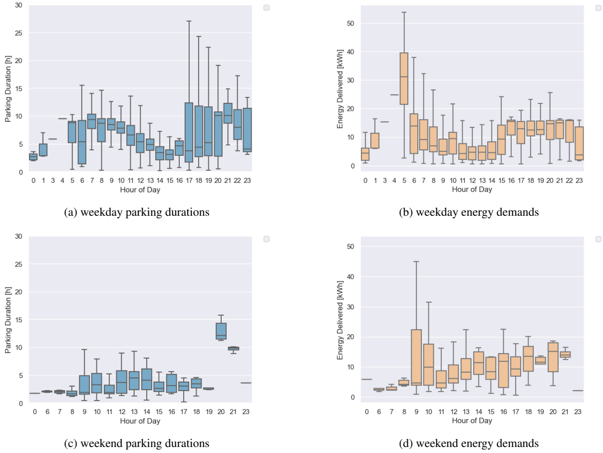
Figure 4: Box plots depicting the distribution of energy delivery and parking duration of EV charging sessions by hour of arrival. Box plots summarize the distribution of data by displaying the median and quantile ranges. Outliers are dismissed for clarity
