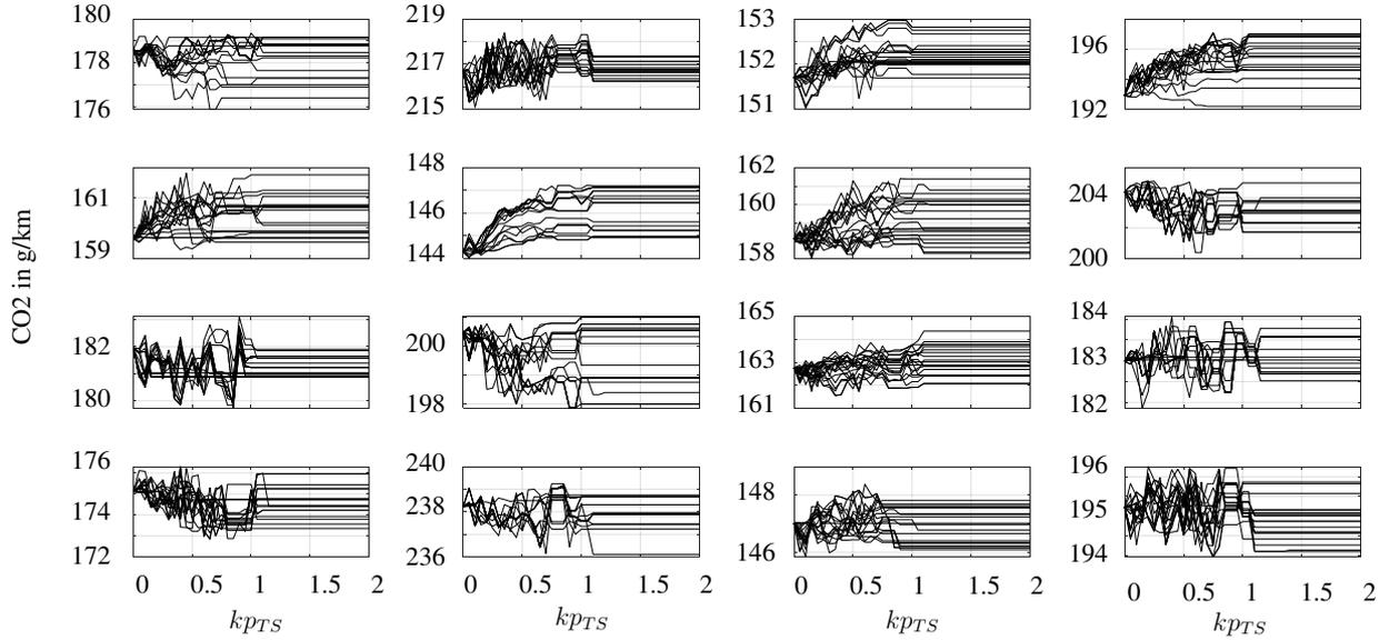
Figure 6: Usable battery energy 25 Wh: CO<sub>2</sub> over  $kp_{TS}$  of several  $t_{horizon}$  for predictive Online ECMS (16/19 cycles). Each graph represents a specific  $t_{horizon}$ .
