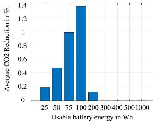
Figure 10: Potentials of the proposed predictive EMS for different usable battery energies: Average CO<sub>2</sub> reduction in % when applying the predictive Online ECMS compared to the non-predictive Online ECMS.
