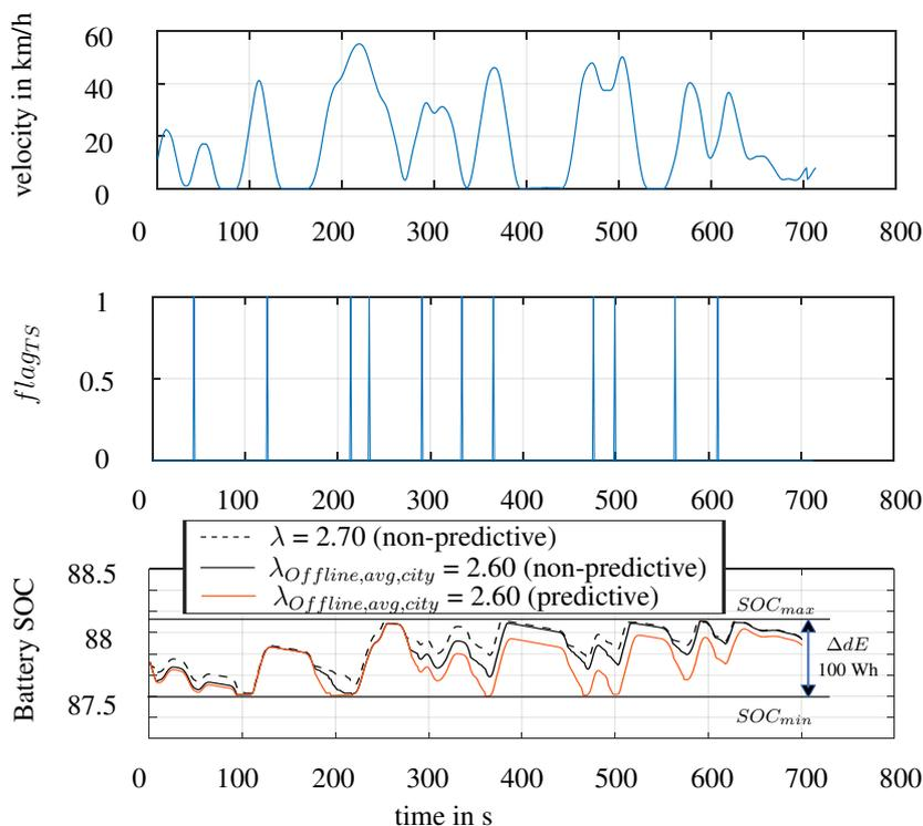
Figure 8: Usable battery energy 100 Wh: Velocity (upper graph),  $flag_{TS}$  (middle graph), and battery SOC over time (lower graph). Both for non-predictive Online ECMS (blue) and predictive Online ECMS (orange) with  $t_{horizon} = 65$  s,  $k_{pTS} = 0.2$ . In addition, the course for the non-predictive Online ECMS with  $\lambda = 2.70$  is plotted.
