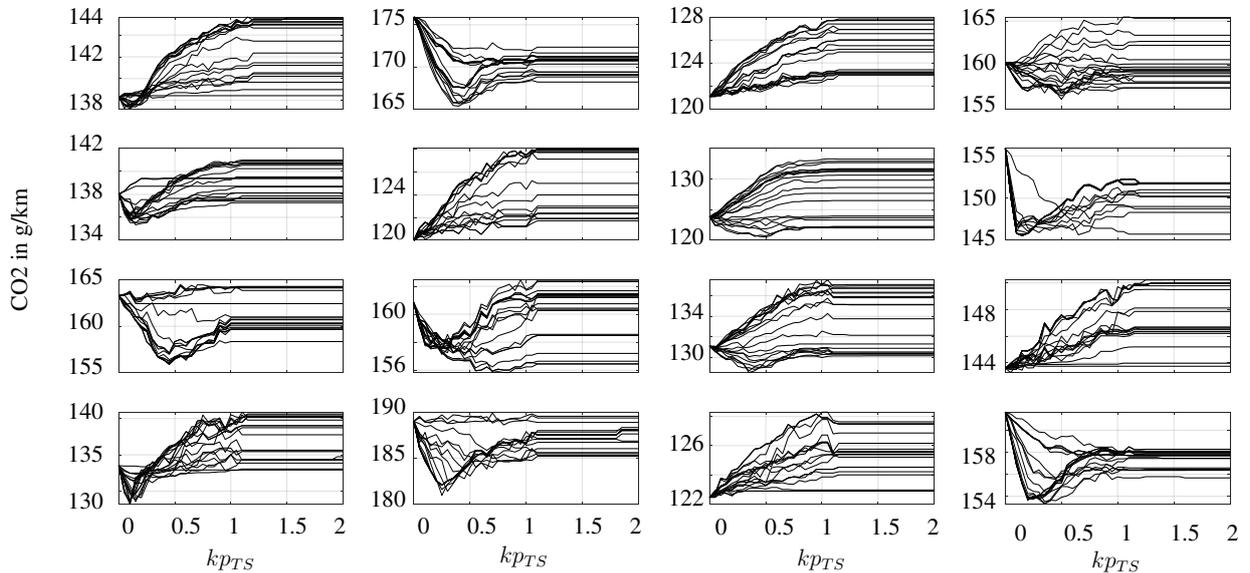
Figure 7: Usable battery energy 100 Wh: CO<sub>2</sub> over  $kp_{TS}$  of several  $t_{horizon}$  for predictive Online ECMS (16/19 cycles). Each graph represents a specific  $t_{horizon}$ .
