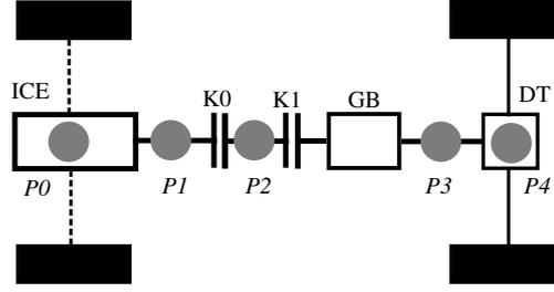
Figure 1: Topologies of HEVs in parallel configuration from [29].
