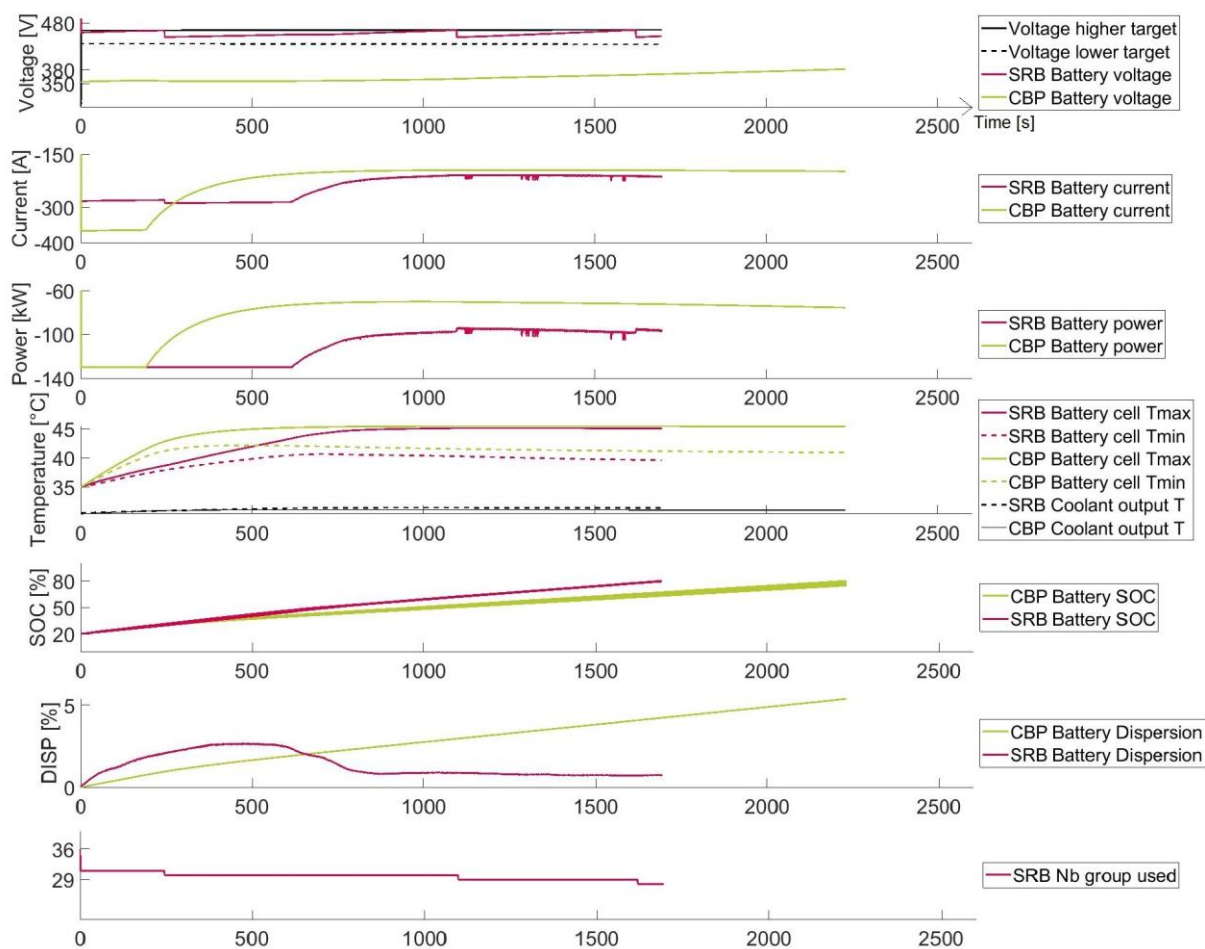
Figure 2 simulation of Fast DC charging for CBP and SRB
